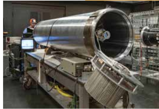
Open shutter door with instrument visible during testing at Wallops. NASA Photo/Berit Bland
