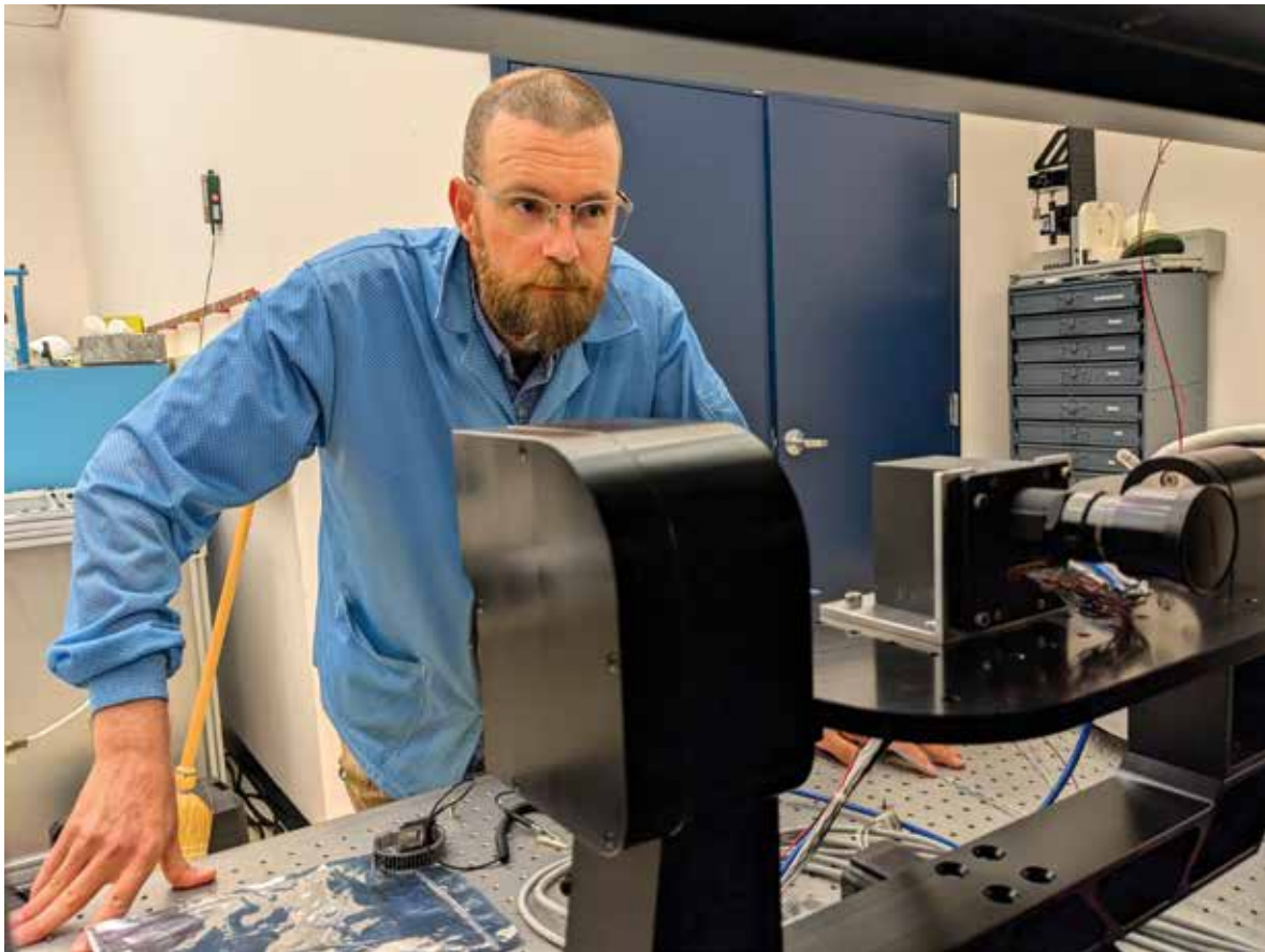
Lens Calibration of the WaIST Prototype Credit: Zach Peterson
