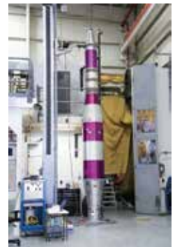
Bend testing of payload. NASA Photo/Berit Bland
